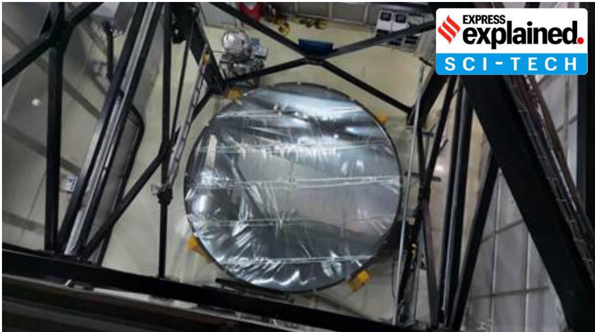
Top view of the ILMT located at the Devasthal Observatory of ARIES showing the liquid mercury mirror covered by a thin mylar film. (PIB)
