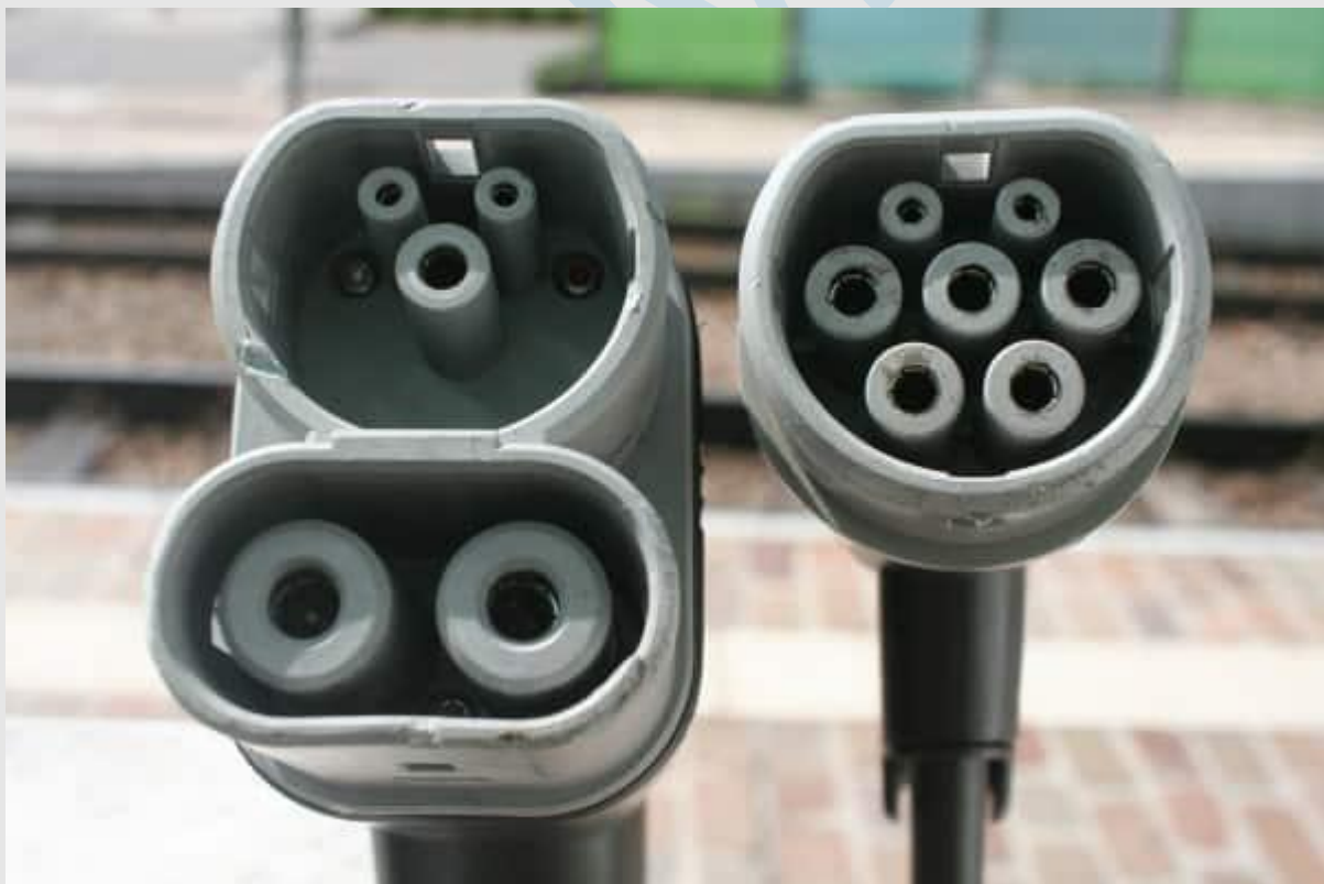
Figure 1 European-style combined charging system (left) and Europe-style Type 2 connector for AC charging and slow DC charging (right).
