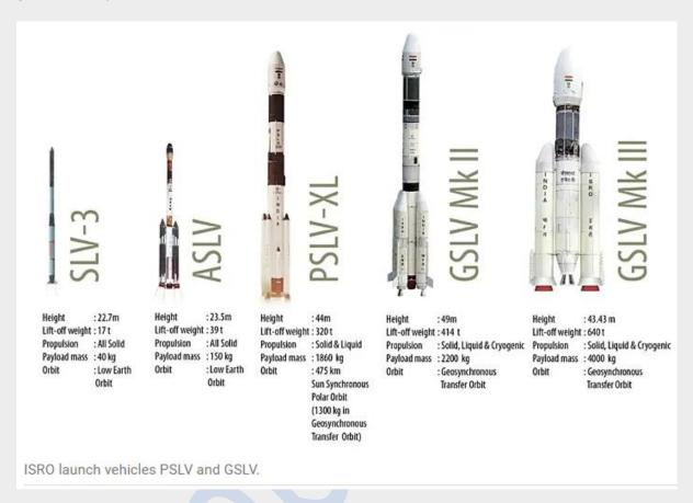
GSLVs have a higher capacity because sending satellites deeper into space requires greater power. Therefore, cryogenic engines consisting of liquid hydrogen and liquid oxygen are used in GSLVs as they provide greater thrust than the engines used in the older launch vehicles. The GSLV Mk-II can carry satellites weighing up to 2,200 kg, while the Mk-III can carry up to 4,000 kg.
