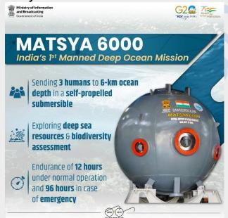
Last month, India completed wet testing of its Matsya-6000 submersible, capable of diving up to 6 km below the surface to look for underwater minerals off the coast. The launch of the first deep-sea manned vehicle is planned for later this year — it will put India in a select group of nations with the capability to send humans to these depths.
