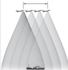
Synthetic-Aperture Radar (SAR) is a form of radar that uses the movement of radar antenna to create a higher resolution images of objects. Such images may be either twodimensional or three-dimensional. SAR uses the motion of the radar antenna over a target region to provide a higher resolution than conventional beam-scanning radars.
