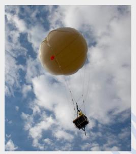
Weather agencies across the world use weather balloons to make upper air observations that are crucial for forecasts. Upper air refers to the Earth's atmosphere above about 5,000 feet, and it is from here that the planet gets its rain and drought, wind and calm, and heat and cold at the surface.
